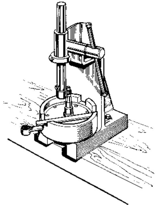
FIG. B14. *Reassembling the flywheels.*
