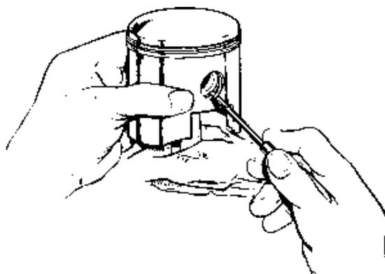
FIG. B4. *Removing circlip*
