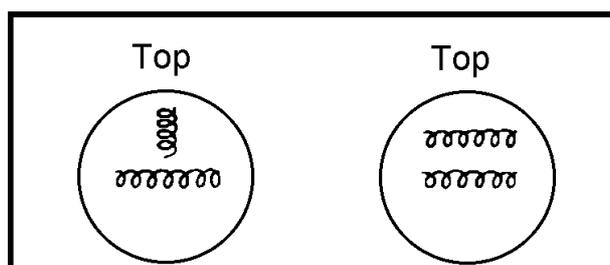
Correct way to fit double-filament bulbs.
